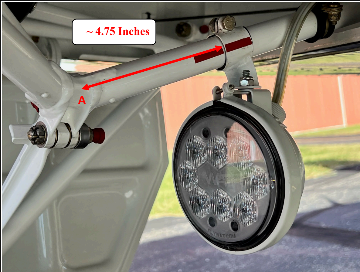
View A (Right Main Landing Gear – Looking Outboard)
